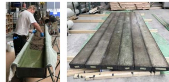
Production of deck profiles with re-used EoL composite
