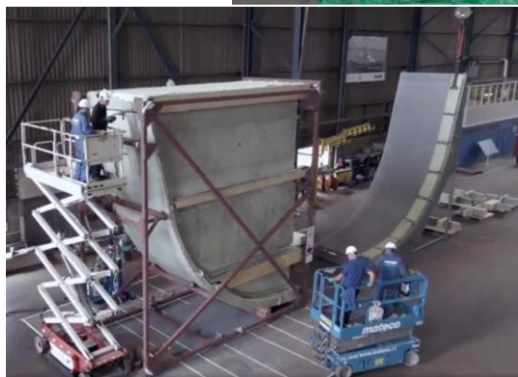
Infused 6m hull section.
