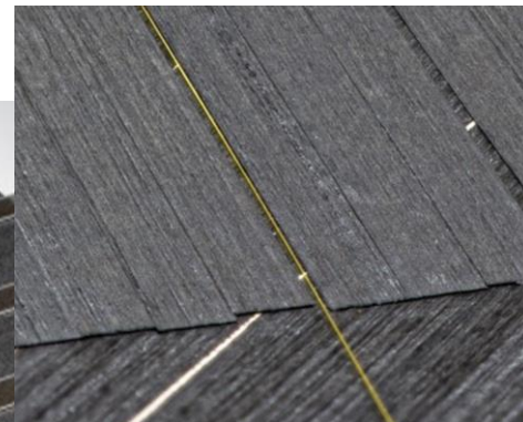
Optical fiber placed with AFP
