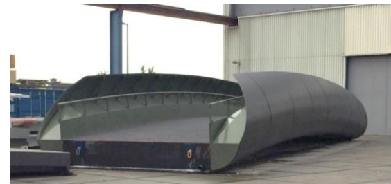
Curved composite sandwich cladding for FiberCore Europe's 21m bridge – 120m 2 weighs < 1000kg.
