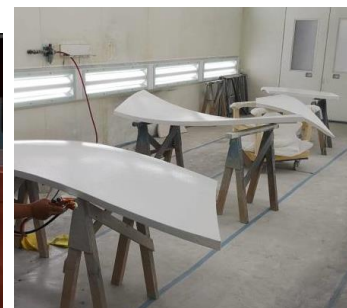
Curve Works FR Tempra panels (rPET core, GF, water-based resin).
