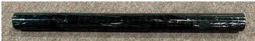
First nanomodified 3R resin tubular demonstrator (June 2020).
