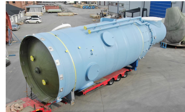
Scrubbers and wash towers Pesureita ja pesutorneja
