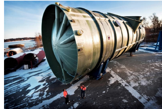
Scrubber dia 8,5 m, 106 tons of composites
