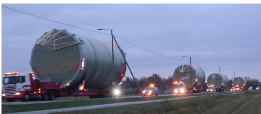
Reactors dia 8m
