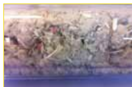
Fig.4 : Typical composite regrind, made from ground windmill blade Courtesy: Zajons, Melbeck
