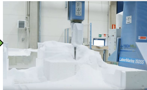
Milling of tooling board
