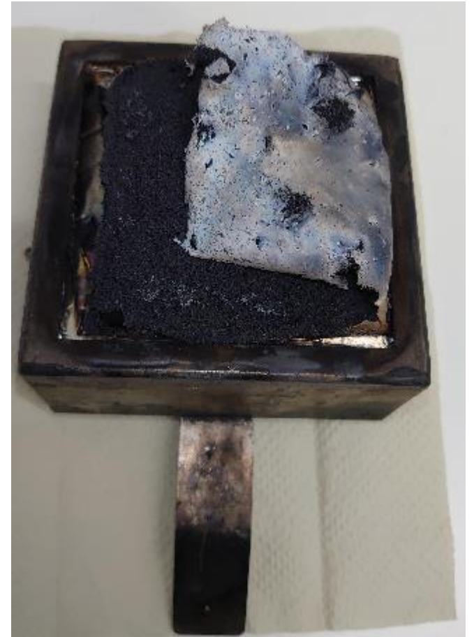
After 20 min burn with 50 kW/m 2
